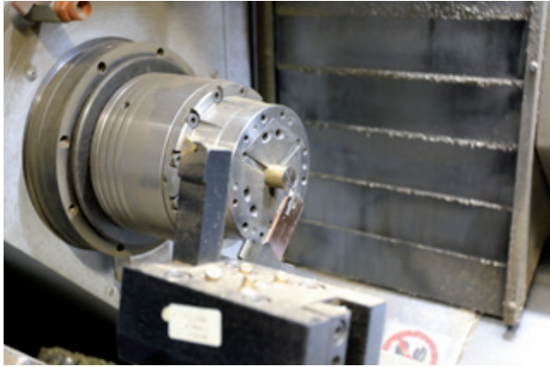
6-sided complete machining: The Hyperturn 65 Powermill is equipped with 5,000 rpm main and counter spindles, a 12,000 rpm BMT turret incl. Y-axis for a maximum of twelve driven tools, and an 18,000 rpm milling spindle with B-axis, enabling the complete machining of various parts made of brass with dry machining in batch sizes down to 1.
