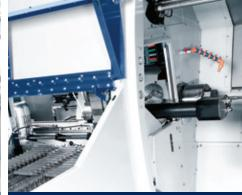
ully automatic shaft loading. Feed-in via a conveyor belt, emoval via the finished parts pick-up device.
