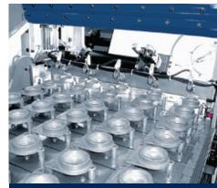
rge storage capacity chain feeding system for loading reformed blanks with the correct orientation.
