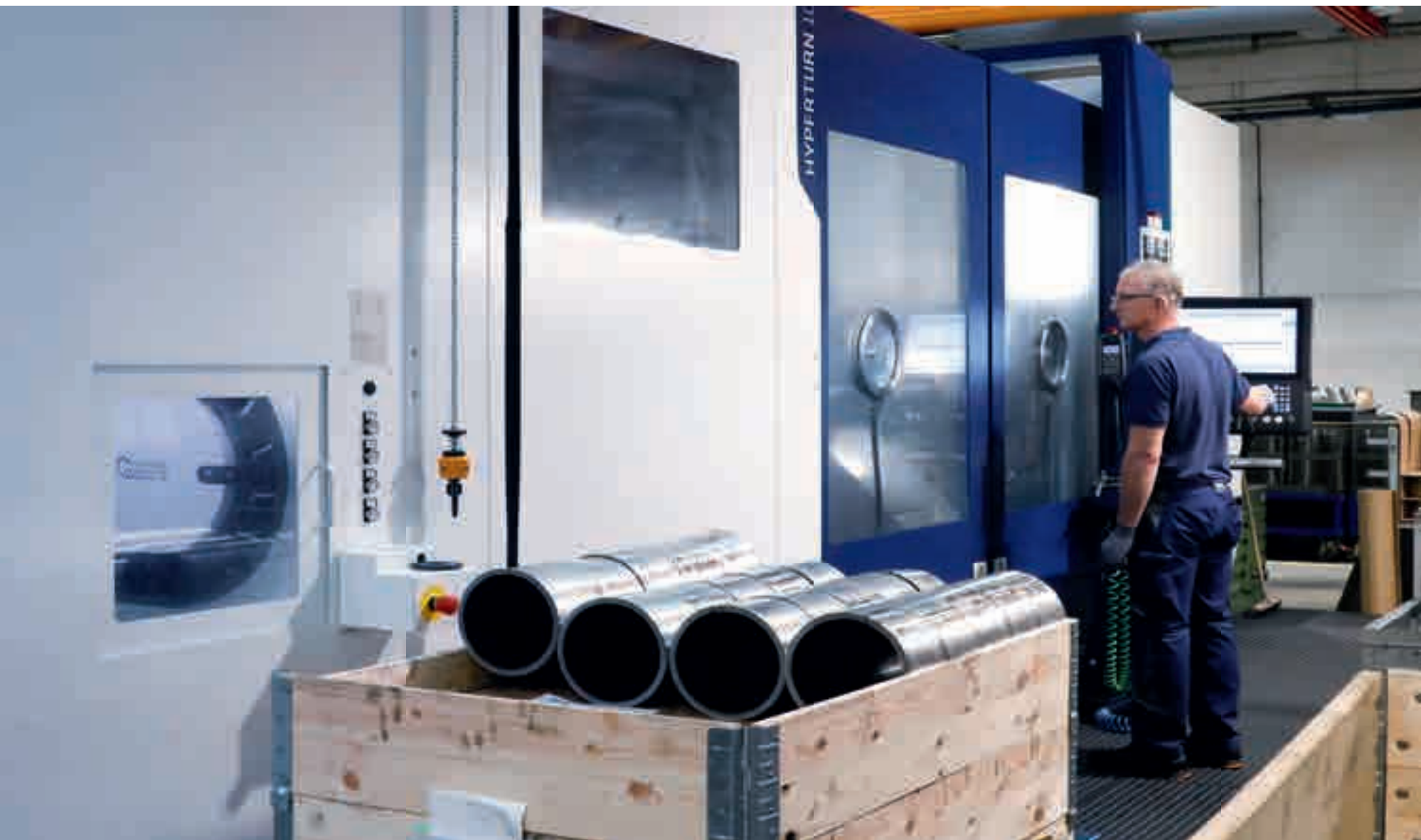
Turn-mill centre HYPERTURN 100 Powermill for complete machining of complex workpieces.
